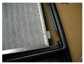
Reinstall the filter, make sure the tabs are to the bottom and are inserted into the slots in the console.
