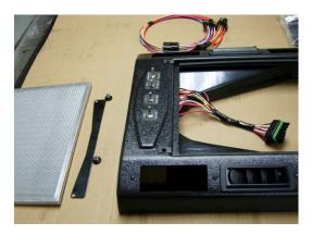
With the filter off you will have access to the wiring harness and will be easier to hook up.
