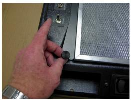
Remove the two thumb screws and the retaining metal hold down - then the filter will slide out of the plastic, there are tabs in the filter opposite of the thumb screws.
