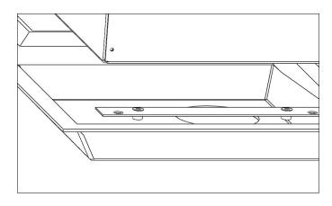
MARK AND CUT OPENINGS FOR AIR INLET AND OUTLET. CAREFULLY DRILL HOLES FOR 8 5/16" MOUNTING BOLTS. PLACE AIR CONDITIONER AND HAND START ALL BOLTS. USE BLUE LOCKTITE OR SIMILAR THREADLOCK (NOT SUPPLIED). NOTE THAT THE 4 BOLTS SURROUNDING THE AIR INLET AND OUTLET PASS THROUGH THE CONSOLE BRACKETS (IF USED). TIGHTEN ALL BOLTS EVENLY TO COMPRESS THE GASKET FROM 3/8" TO APPROXIMATELY 1/4". OVERCOMPRESSING THE GASKET WILL CAUSE LEAKS.
